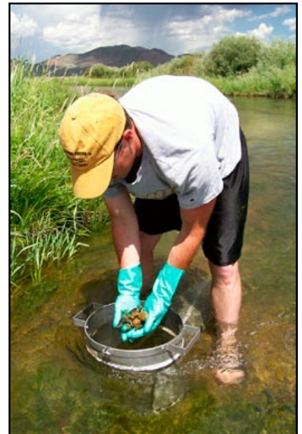
Environmental Science graduate student Nick Whitaker using a Hess sampler to collect macroinvertebrates from Silver Creek.
