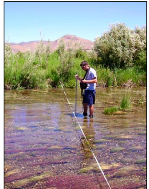
Environmental Science graduate student McClure Tosch measuring the width and depth of a stream channel.
