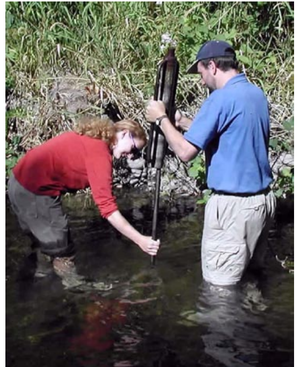
John Selker and Starr Metcalf installing a temperature profiler in the Walla Walla River at Milton Freewater to assess stream aquifer interactions.
